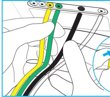
**TIP:** To disconnect, push the coloured connector in to the machine, and gently pull the tube out.
